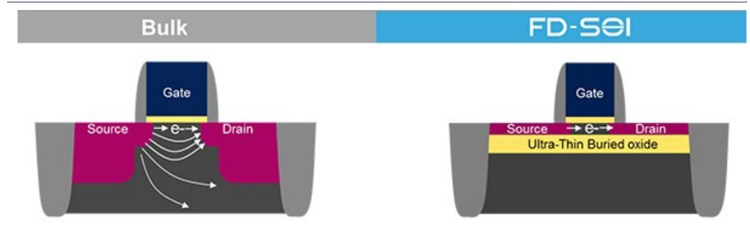
Fig. 6: Cross section of a transistor on bulk wafer vs. FD-SOI
