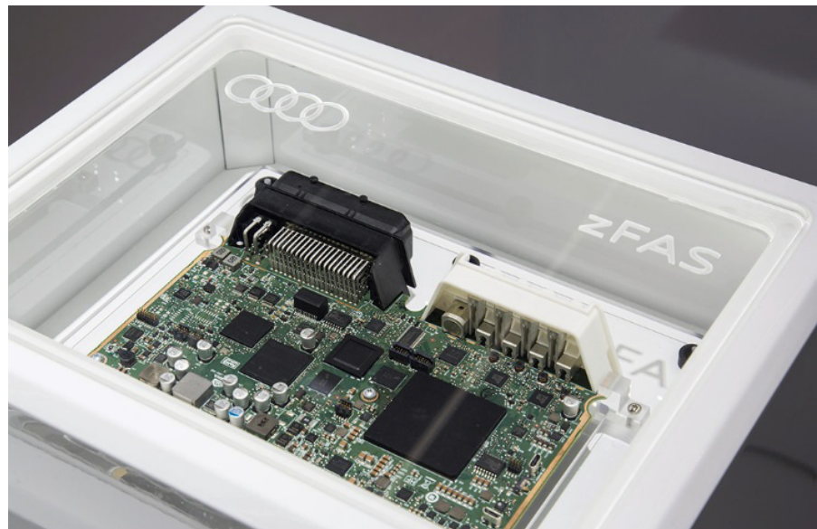
Fig. 18: Audi zFAS system using Mobileye's EyeQ3
