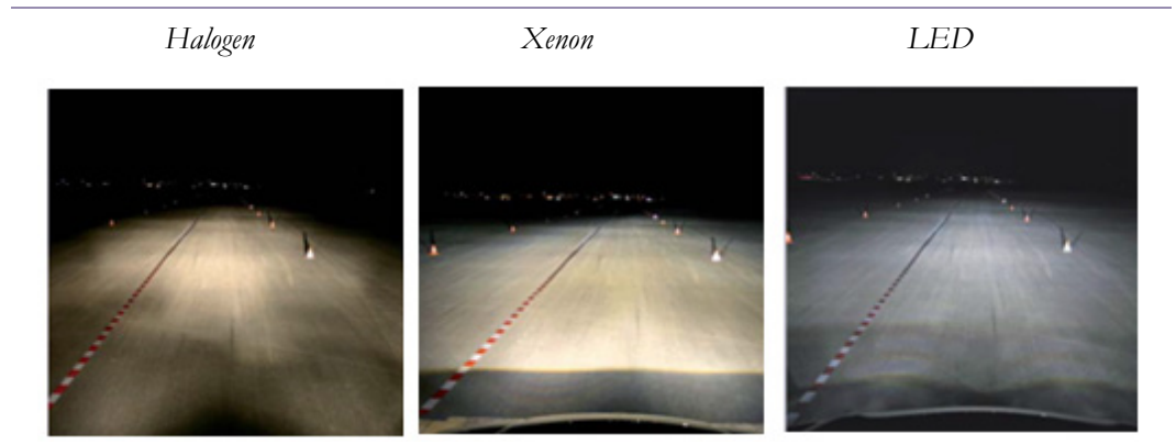
Fig. 7: Luminosity differences depending on technology used
